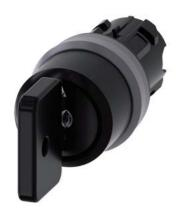
Key-operated switch O.M.R, 22 mm, round, plastic with metal front ring, lock number 73034, black, with 2 keys, 3 switch positions I-O-II, latching, actuating angle 2x45°, 10:30h/12h/13:30h, Key removal I+O+II, Z=50-unit packaging
