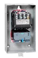
Non-reversing motor starter, Size 1, Three phase full voltage, Solid-state overload relay, OLR amp range 10-40A, 110V 50Hz / 120V 60Hz coil, Non-combination type, Enclosure type 1, Indoor general purpose use, Extra-wide enclosure
