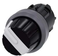
Selector switch, 22 mm, round, plastic with metal front ring, white, Rotary knob, 4 switch positions I-II-III-IV, latching, Actuating angle 4x90°, 3h/6h/9h/12h, with laser labeling, inscription or symbol Customer-specific selection with SIRIUS ACT configurator (CIN)
