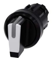
Selector switch, illuminable, 22 mm, round, plastic, white, selector switch, short, 3 switch positions I>O<II, momentary contact on the left, latching on the right, actuating angle 2x45°, 10:30h/12h/13:30h, with laser labeling, inscription or symbol Customer-specific selection with SIRIUS ACT configurator (CIN)
