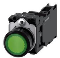
Illuminated pushbutton, 22 mm, round, plastic, green, pushbutton, flat, momentary contact type, with holder, 1 NO+1 NC, LED module with integrated LED 24 V AC/DC, spring-type terminal, with laser labeling, symbol number according to, ISO 7000 or IEC 60417
