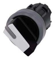
Selector switch, illuminable, 22 mm, round, plastic with metal front ring, white, selector switch, short, 2 switch positions O<I, momentary contact type, Actuating angle 45°, 10:30h/12h, Z=50-unit packaging
