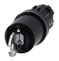
Key-operated switch IKON, 22 mm, round, plastic, lock number 360012K1, with 2 keys, 3 switch positions I-O<II, left latching, right momentary contact type, actuating angle  $2\times45^{\circ}$ , 10:30h/12h/13:30h, key removal O+I, with laser labeling, lower case
