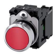
Pushbutton, 22 mm, round, metal, shiny, red, pushbutton, flat, momentary contact type, with holder, 1 NO, screw terminal, with laser labeling, lower case
