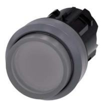
Illuminated pushbutton, 22 mm, round, plastic with metal front ring, clear, pushbutton, raised momentary contact type, with laser labeling, upper case and lower case, always upper case at beginning of line
