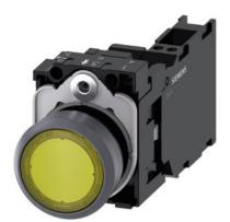
Illuminated pushbutton, 22 mm, round, plastic with metal front ring, yellow, pushbutton, flat, momentary contact type, with holder, 1 NO+1 NC, LED module with integrated LED 24 V AC/DC, spring-type terminal, with laser labeling, upper case
