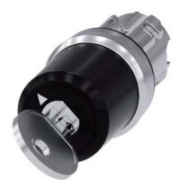
key-operated switch Siemens, 22 mm, round, metal, shiny, lock number SSG10, with 2 keys, 2 switch positions O<I, momentary contact type, actuating angle 45°, 10:30h/12h, key removal O, Z=50-unit packaging
