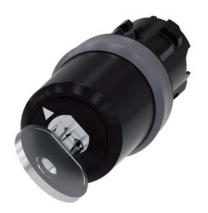
Key-operated switch BKS, 22 mm, round, plastic with metal front ring, Lock No. E7 (VW), without key, 2 switch positions O-I, latching, actuating angle 90°, 10:30h/13:30h, key removal O+I, with laser labeling, upper case and lower case, always upper case at the beginning of the word
