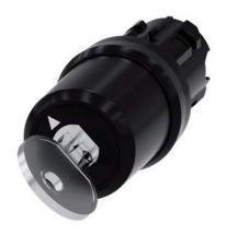
key-operated switch Siemens, 22 mm, round, plastic, special lock, with 2 keys, 2 switch positions O-I, latching, actuating angle  $90^\circ$ , 10:30h/13:30h, key removal O+I
