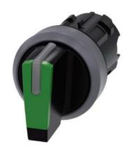
Selector switch, illuminable, 22 mm, round, plastic with metal front ring, green, selector switch, short, 3 switch positions I>O<II, momentary contact type, actuating angle 2x45°, 10:30h/12h/13:30h, with laser labeling, inscription or symbol Customer-specific selection with SIRIUS ACT configurator (CIN)
