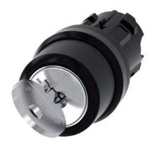
RONIS key-operated switch, 22 mm, round, plastic, lock number 455, with 2 keys, 2 switch positions O<I, momentary contact type, Actuating angle 45°, 10:30h/12h, key removal O, with laser labeling, upper case
