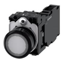
Illuminated pushbutton, 22 mm, round, plastic, clear, pushbutton, flat, momentary contact type, with holder, 1 NO+1 NC, LED module with integrated LED 110 V AC, screw terminal, with laser labeling, lower case
