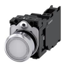
Illuminated pushbutton, 22 mm, round, metal, shiny, white, pushbutton, flat, momentary contact type, with holder, 1 NO+1 NC, LED module with integrated LED 110 V AC, spring-type terminal, with laser labeling, upper case
