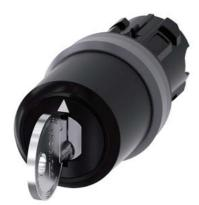
Key-operated switch IKON, 22 mm, round, plastic with metal front ring, lock number 360012K1, with 2 keys, 3 switch positions I-O<II, left latching, right momentary contact type, actuating angle 2x45°, 10:30h/12h/13:30h, key removal O+I, with laser labeling, upper case
