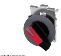
Selector switch, illuminable, 30 mm, round, Metal, matte, red, selector switch, long, front ring for flush installation, 2 switch positions O-I, latching, actuating angle 90°, 10:30h/13:30h, with laser labeling, inscription or symbol Customer-specific selection with SIRIUS ACT configurator (CIN)
