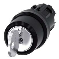
RONIS key-operated switch, 22 mm, round, plastic, lock number SB30, with 2 keys, 3 switch positions I-O-II, latching, actuating angle 2x45°, 10:30h/12h/13:30h, Key removal II, possible special locks: SB31, 421, 455, with laser labeling, upper case and lower case, always upper case at beginning of line
