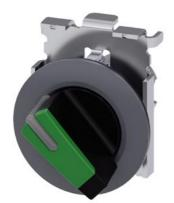
Selector switch, illuminable, 30 mm, round, Metal, matte, green, selector switch, short, front ring for flush installation, 2 switch positions O<I, momentary contact type, Actuating angle 45°, 10:30h/12h, with laser labeling, upper case and lower case, always upper case at the beginning of the word
