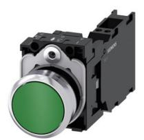
Pushbutton, 22 mm, round, metal, shiny, green, pushbutton, flat, momentary contact type, 1 NO+1 NC, spring-type terminal, with laser labeling, upper case and lower case, always upper case at the beginning of the word
