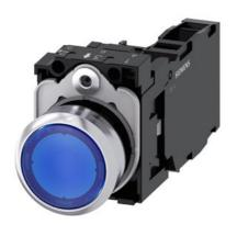
Illuminated pushbutton, 22 mm, round, metal, shiny, blue, pushbutton, flat, momentary contact type, with holder, 1 NO+1 NC, LED module with integrated LED 24 V AC/DC, screw terminal, with laser labeling, lower case
