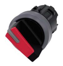
Selector switch, illuminable, 22 mm, round, plastic with metal front ring, red, selector switch, short, 2 switch positions O<I, momentary contact type, Actuating angle 45°, 10:30h/12h, Z=50-unit packaging
