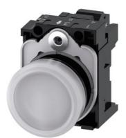
Indicator lights, 22 mm, round, plastic, white, lens, smooth, with holder, LED module, with integrated LED 110 V AC, spring-type terminal, with laser labeling, upper case
