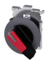
Selector switch, illuminable, 30 mm, round, Metal, matte, red, selector switch, long, front ring for flush installation, 2 switch positions O<I, momentary contact type, Actuating angle 45°, 10:30h/12h, with laser labeling, upper case and lower case, always upper case at beginning of line
