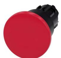
Mushroom pushbutton, 22 mm, round, plastic, red, 40mm, latching, pull-tounlatch mechanism, Z=50-unit packaging
