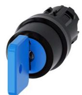
Key-operated switch O.M.R, 22 mm, round, plastic, lock number 73038, blue, with 2 keys, 3 switch positions I-O-II, latching, actuating angle 2x45°, 10:30h/12h/13:30h, key removal O, with laser labeling, lower case
