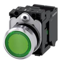
Illuminated pushbutton, 22 mm, round, metal, shiny, green, pushbutton, flat, momentary contact type, with holder, 1NO, LED module with integrated LED 24 V AC/DC, spring-type terminal, with laser labeling, upper case and lower case, Always upper case at the beginning of the word
