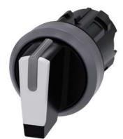
Selector switch, illuminable, 22 mm, round, plastic with metal front ring, white, selector switch, short, 3 switch positions I>O<II, momentary contact type, actuating angle  $2x45^{\circ}$ , 10:30h/12h/13:30h, Z=50-unit packaging
