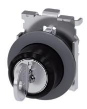
RONIS key-operated switch, 30 mm, round, Metal, matte, front ring for flush installation, lock number SB30, with 2 keys, 3 switch positions I-O-II, latching, actuating angle 2x45°, 10:30h/12h/13:30h, Key removal I+O+II, possible special locks: SB31, 421, 455, with laser labeling, upper case and lower case, always upper case at beginning of line
