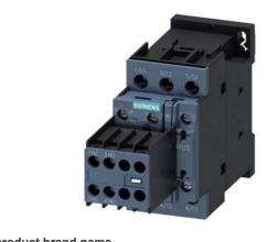
power contactor, AC-3 25 A, 11 kW / 400 V 2 NO + 2 NC, 110 V AC, 50 Hz, 3-pole, Size S0 screw terminal Removable auxiliary switch
