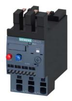
Overload relay 1.8...2.5 A Thermal For motor protection Size S0, Class 10 Contactor mounting Main circuit: Spring-type terminal Auxiliary circuit: spring-type terminal Manual-Automatic-Reset
