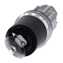
Key-operated switch IKON, 22 mm, round, metal, shiny, lock number 360012K1, with 2 keys, 2 switch positions O-I, latching, actuating angle 90°, 10:30h/13:30h, key removal O, with laser labeling, upper case and lower case, always upper case at beginning of line
