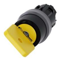
Key-operated switch O.M.R, 22 mm, round, plastic with metal front ring, lock number 73033, yellow, with 2 keys, 2 switch positions O-I, latching, actuating angle 90°, 10:30h/13:30h, key removal O, Z=50-unit packaging
