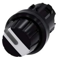
Selector switch, illuminable, 22 mm, round, plastic, white, Rotary knob, 2 switch positions O-I, latching, actuating angle 90°, 10:30h/13:30h, with laser labeling, inscription or symbol Customer-specific selection with SIRIUS ACT configurator (CIN)
