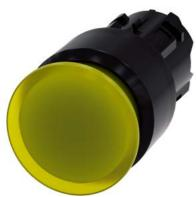
Illuminated mushroom pushbutton, 22 mm, round, plastic, yellow, 30 mm, latching, pull-to-unlatch mechanism, with laser labeling, symbol number according to, ISO 7000 or IEC 60417
