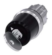
key-operated switch Siemens, 22 mm, round, metal, shiny, lock number SSG10, with 2 keys, 2 switch positions O-I, latching, actuating angle 90°, 10:30h/13:30h, key removal O+I, with laser labeling, upper case and lower case, always upper case at beginning of line
