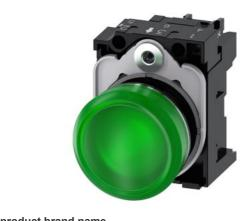
Indicator lights, 22 mm, round, metal, shiny, green, lens, smooth, with holder, LED module with integrated LED 230 V AC, screw terminal, Z=20-unit packaging
