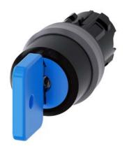
Key-operated switch O.M.R, 22 mm, round, plastic with metal front ring, lock number 73038, blue, with 2 keys, 3 switch positions I-O-II, latching, actuating angle 2x45°, 10:30h/12h/13:30h, Key removal I+O+II, with laser labeling, upper case and lower case, always upper case at beginning of line
