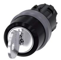
RONIS key-operated switch, 22 mm, round, plastic with metal front ring, lock number SB30, with 2 keys, 3 switch positions I-O<II, left latching, right momentary contact type, actuating angle 2x45°, 10:30h/12h/13:30h, key removal O+I, possible special locks: SB31, 421, 455, with laser labeling, upper case
