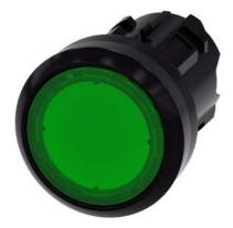
Illuminated pushbutton, 22 mm, round, plastic, green, pushbutton, flat, latching, Push-to-release mechanism, with laser labeling, inscription or symbol Customer-specific selection with SIRIUS ACT configurator (CIN)
