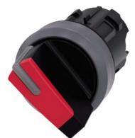
Selector switch, illuminable, 22 mm, round, plastic with metal front ring, red, selector switch, short, 2 switch positions O<I, momentary contact type, Actuating angle 45°, 10:30h/12h, with laser labeling, upper case
