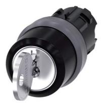
RONIS key-operated switch, 22 mm, round, plastic with metal front ring, lock number SB30, with 2 keys, 3 switch positions I>O<II, momentary contact on the left, latching on the right, actuating angle 2x45°, 10:30h/12h/13:30h, key removal O, possible special locks: SB31, 421, 455, with laser labeling, upper case
