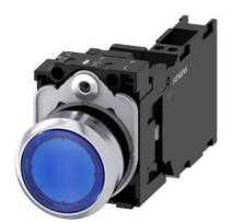
Illuminated pushbutton, 22 mm, round, metal, shiny, blue, pushbutton, flat, momentary contact type, with holder, 1 NO+1 NC, LED module with integrated LED 24 V AC/DC, spring-type terminal, with laser labeling, upper case
