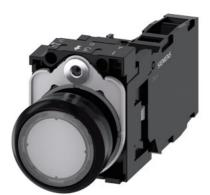
Illuminated pushbutton, 22 mm, round, plastic, clear, pushbutton, flat, momentary contact type, with holder, 1 NO+1 NC, LED module with integrated LED 24 V AC/DC, screw terminal, with laser labeling, inscription or symbol Customer-specific selection with SIRIUS ACT configurator (CIN)
