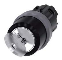
RONIS key-operated switch, 22 mm, round, plastic with metal front ring, lock number SB30, with 2 keys, 2 switch positions O-I, latching, actuating angle 90°, 10:30h/13:30h, key removal O, possible special locks: SB31, 421, 455, with laser labeling, inscription or symbol Customer-specific selection with SIRIUS ACT configurator (CIN)
