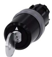
key-operated switch Siemens, 22 mm, round, plastic with metal front ring, special lock, with 2 keys, 3 switch positions I-O-II, latching, actuating angle 2x45°, 10:30h/12h/13:30h, key removal O+I
