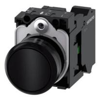
Pushbutton, 22 mm, round, plastic, black, pushbutton, flat, momentary contact type, with holder 1 NO, spring-type terminal, with laser labeling, symbol number according to, ISO 7000 or IEC 60417
