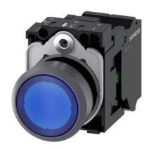
Illuminated pushbutton, 22 mm, round, plastic with metal front ring, blue, pushbutton, flat, momentary contact type, with holder, 1NO, LED module with integrated LED 24 V AC/DC, spring-type terminal, with laser labeling, symbol number according to, ISO 7000 or IEC 60417
